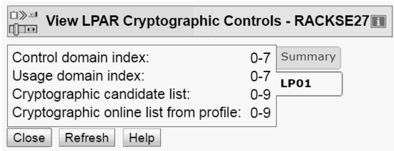
Figure 64. View LPAR cryptographic controls (showing tab containing crypto configuration information for an active partition)
